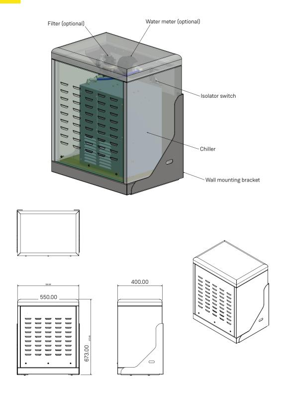
Note: The remote chiller housing is compatible with the Aquafil Remote Chiller. (Refer to separate specification sheet for chiller specifications)
